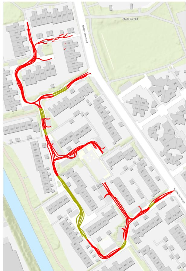
FIGURE 3. Applied pavement materials (red = concrete pavers, green = concrete paving slabs).
