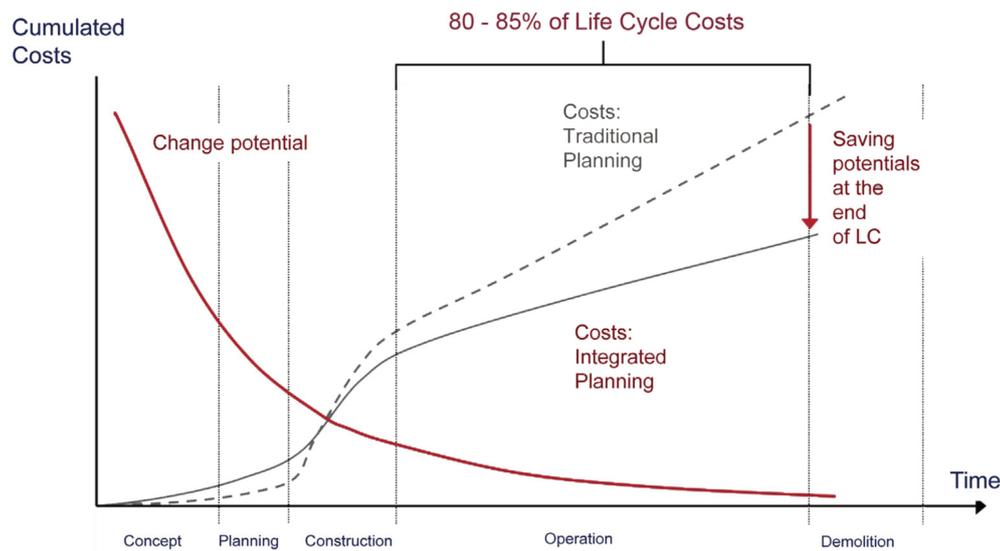
FIGURE 2. Cost development vs. change potential over building life cycle [5].
