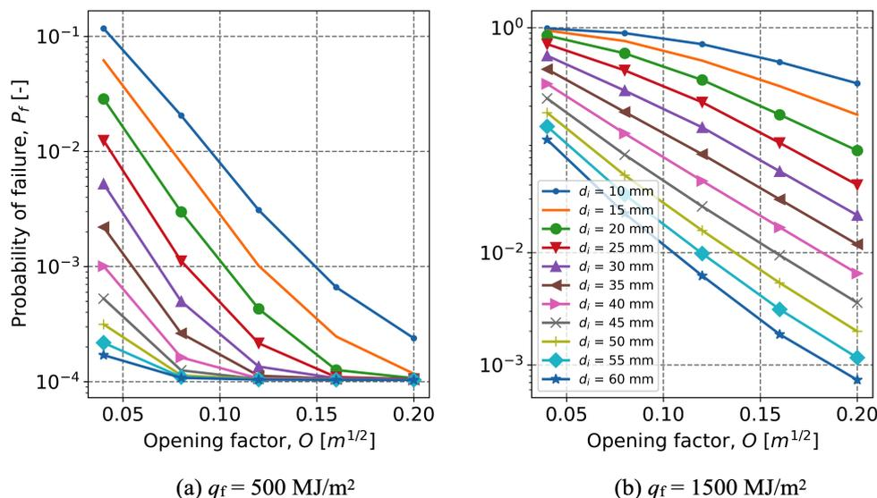
FIGURE 2. Fragility curves for steel columns with varying SFRM thickness under parametric fire exposure.
