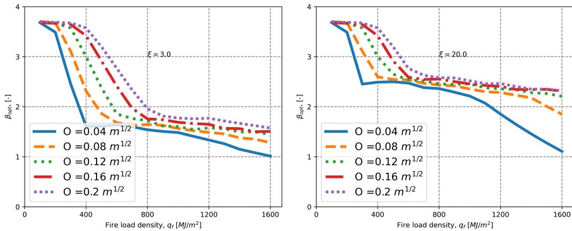
FIGURE 5. Reliability targets for steel column for parametric fire exposure of steel column (constant annual fire probability of  $2.5 \times 10^{-3}$  and, two cases of relative failure costs,  $\xi = 3.0$  and  $20.0$  considered).
