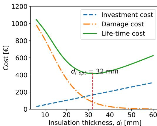
FIGURE 3. Investment, failure and life-time cost for a specific fire scenario case of steel column ( $q_f = 800 \text{ MJ/m}^2$  and  $O = 0.04 \text{ m}^{1/2}$ ). Optimum SFRM thickness,  $d_{i,opt}$  of 32 mm obtained for the case.
