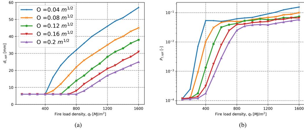
FIGURE 4. Optimum (a) SFRM thicknesses and (b) failure probability for considered cases of fire scenarios of steel column.
