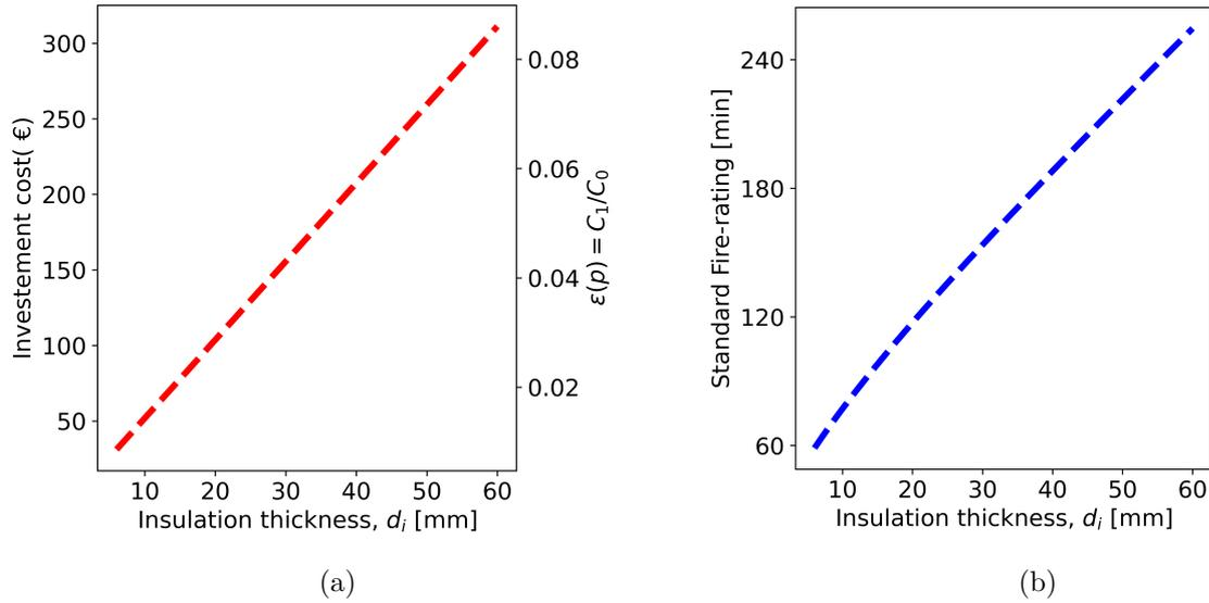
FIGURE 1. (a) Cost of SFRM insulation of steel column. (b) Relationship between SFRM insulation thickness and standard fire-rating of the steel column (based on ISO 834 criteria)
