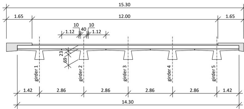
FIGURE 2. Section of bridge structure 29/1.
