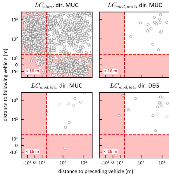
FIGURE 8. Spatial gaps of vehicles on fast lane to adjacent vehicles in slow lane, for different lane configurations.
