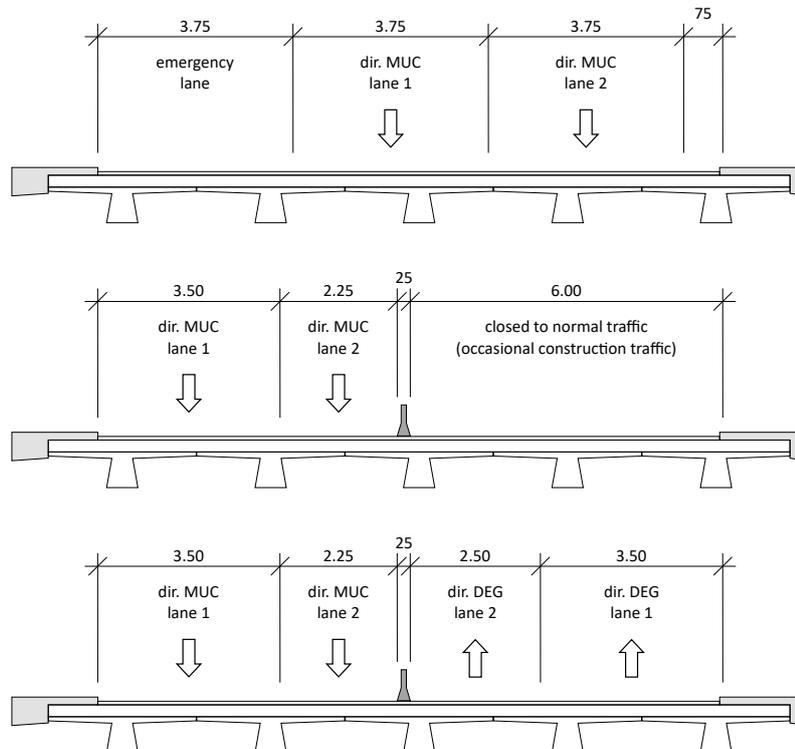
FIGURE 3. Lane configurations  $LC_{stan}$  (top),  $LC_{mod,uni2}$  (middle), and  $LC_{mod,bi4}$  (bottom).
