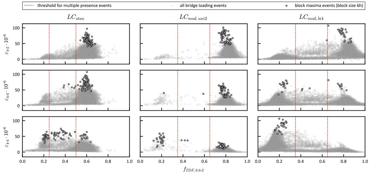
FIGURE 10. TDFs  $f_{TDF,k|4-2}$  evaluated for all BLEs identified from structural monitoring data of working days (BM events with blocks size 6 h highlighted), for different lane configurations and considered response-sensors.
