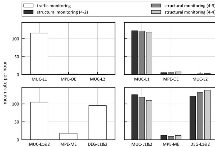
FIGURE 11. Mean hourly occurrence rates of different BLE types for lane configurations  $LC_{stan}$  and  $LC_{mod,bi4}$ , evaluated for working days.
