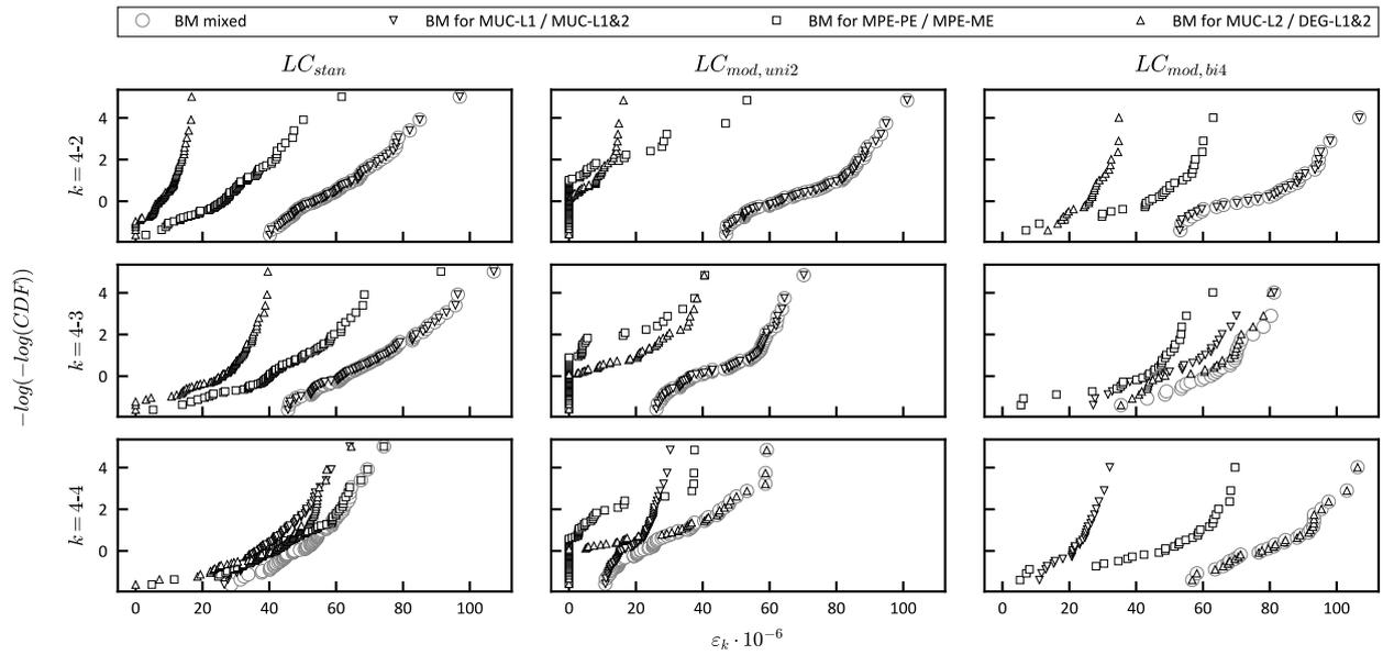
FIGURE 12. BM data (block size 6 h) of working days for considered sensors and different lane configurations; with and without differentiation of different BLE types.
