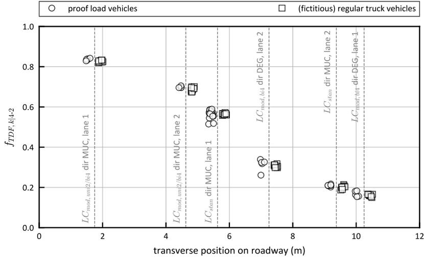
FIGURE 6. TDFs  $f_{TDF,k|4-2}$  from proof load testing and evaluation of regular truck vehicles with reference influence line (RIL).
