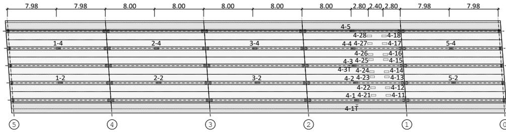
FIGURE 4. Overview of sensor layout of structural monitoring at bridge structure 29/1.
