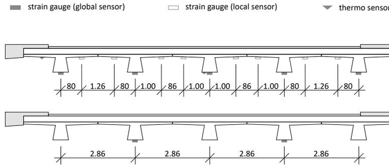
FIGURE 5. Sensor locations within bridge section of span no. 4 (top) and remaining spans (bottom).
