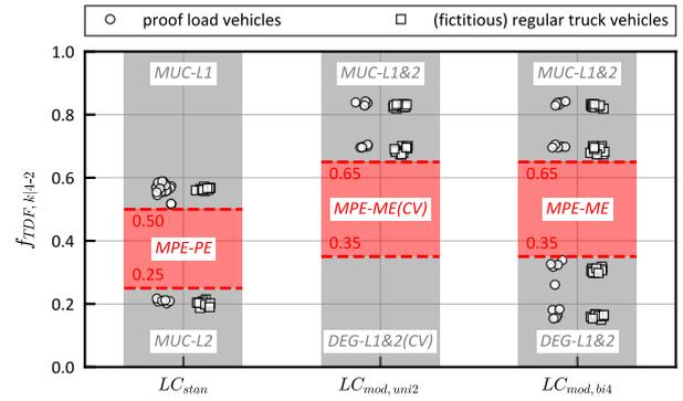
FIGURE 9. Definition of threshold values for MPE identification for different lane configurations.
