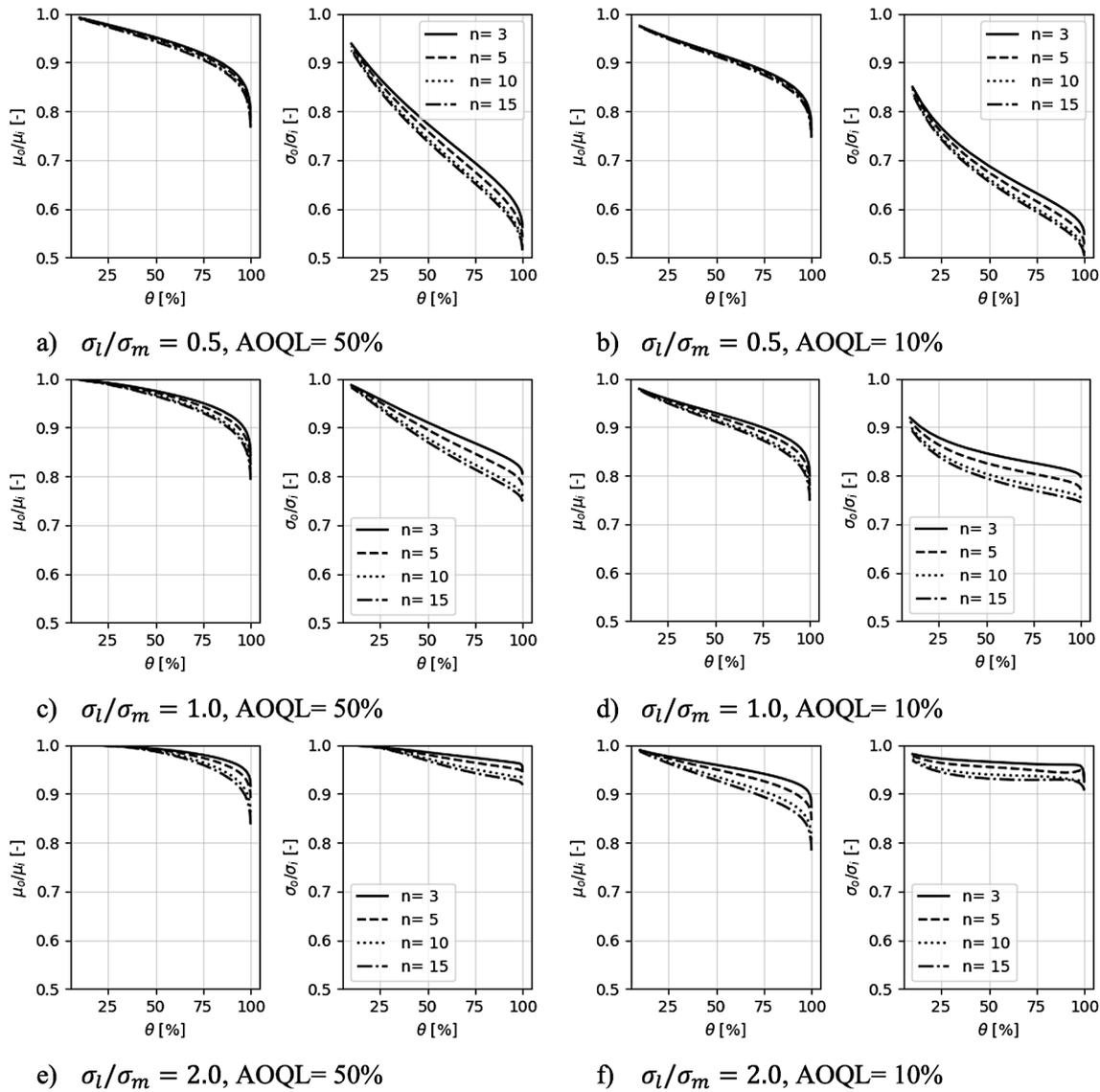
FIGURE 4. Filter effect based on  $\bar{x}_n \leq D_m + \lambda \sigma_i$  (AOQL= 50%) or  $\bar{x}_n \leq D_k + \lambda \sigma_i$  (AOQL= 10%) with  $\sigma_i = 0.1D_m$ .
