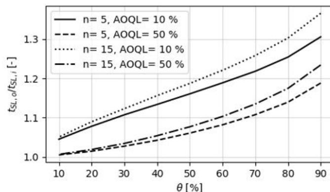
FIGURE 5. Influence of conformity control on the initiation period and on the service life.
