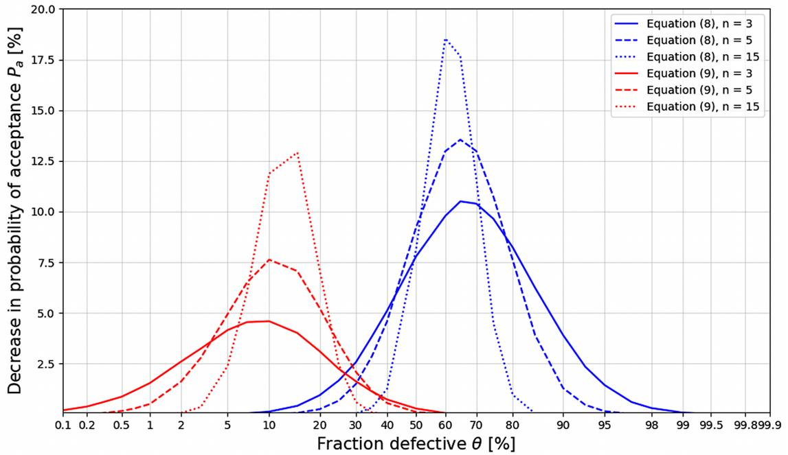
FIGURE 2. Decrease in probability of accepting a concrete batch when going from 2 tests with  $n$  different samples to  $n + 1$  tests with a moving average (AOQL= 50% and  $\bar{x}_n \leq D_m + \lambda s_n$ ).
