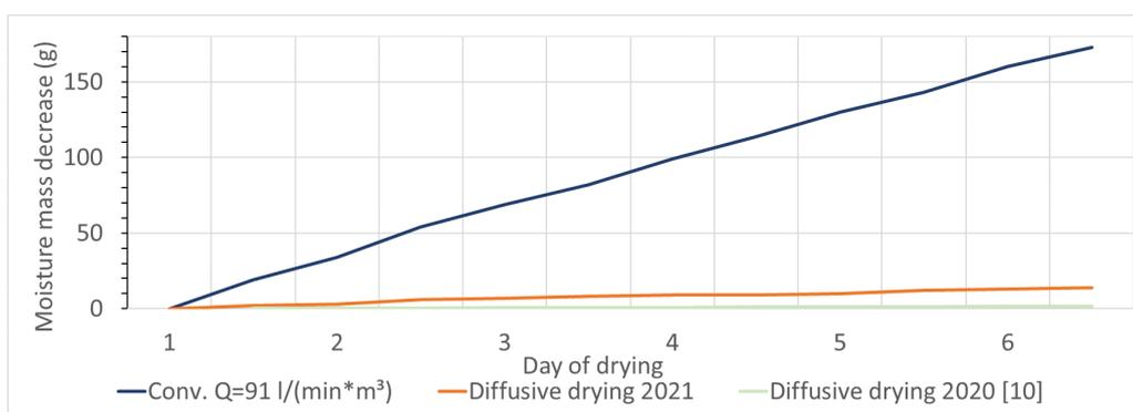
FIGURE 4. Moisture dry-out at stable temperature conditions (Figure 1). Diffusive drying 2020 refers to a previous research on vapour retarding and vapour permeable tape performance [9].
