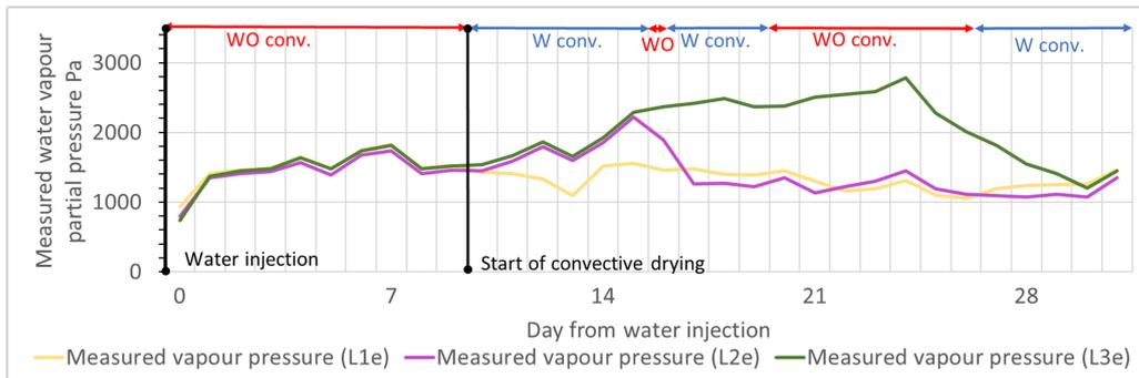
FIGURE 6. Daily running average of measured water vapour pressures in convective drying wall section.
