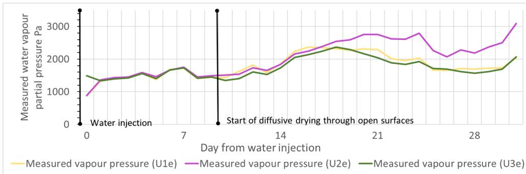
FIGURE 5. Daily running average of measured water vapour pressures in diffusive drying wall section.
