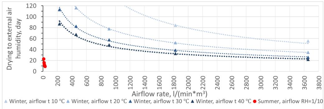
FIGURE 7. Moisture dry-out duration at stable temperature conditions to outside air humidity (pore air vapour content in summer  $9.3/10 = 0.93 \text{ (g/m}^3\text{)}$  and in winter  $3.3 \text{ (g/m}^3\text{)}$ ). Blue lines indicate drying in winter at different air inflow temperatures, red line shows drying in summer with reduced moisture content in the air.
