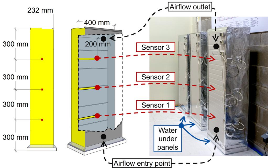
FIGURE 1. 3D mock-up test elements: (a) with indicated T and RH sensor placement (red dots, Hobo UX-100-023), airflow sensors (black dots SMC PFM 710) and photos of the elements (b).
