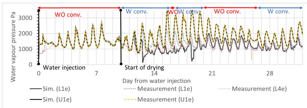
FIGURE 3. Modelled water vapour pressure at sensor positions compared to measured results (Figure 2). W conv. is for time range when lower section of the wall was ventilated and WO conv. when not.
