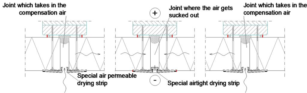
FIGURE 10. Scheme on top view of facade for ventilated vertical joints and compensation air joints.
