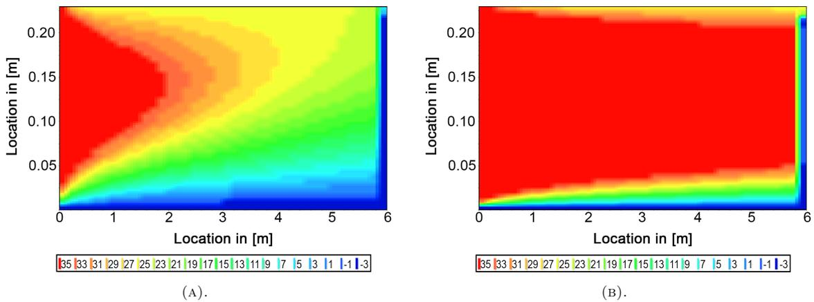
FIGURE 8. Temperature distribution on top view of the wall (vertical length 0.23 m and horizontal length 6 m), winter period, air inflow temperature +40 °C (A) airflow rate 228 l/(min · m³) (B) airflow rate 3650 l/(min · m³). Red area shows temperature over +35 °C and navy blue is for areas under -3 °C.
