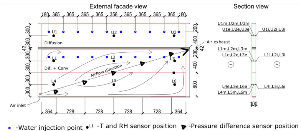
FIGURE 2. Full scale test walls and sensor positioning (T/RH Humisense A1, airflow SMC PFM 725).
