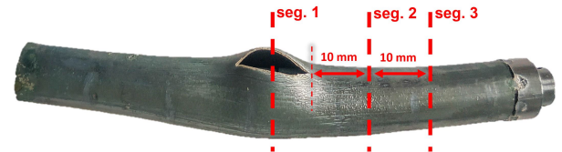
FIGURE 8. Ring segments cut for microscopy analysis.
