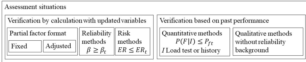
FIGURE 1. Quantitative and qualitative methods to verify the reliability of existing structures.
