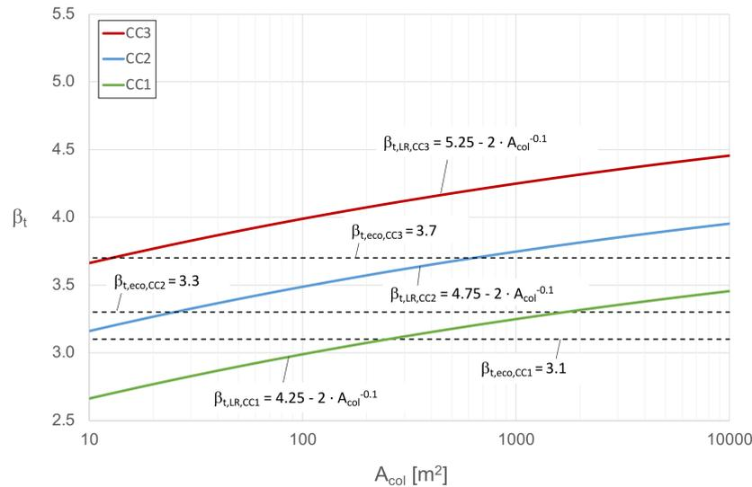
FIGURE 4. Annual reliability requirements for human safety,  $\beta_{t,LR}$ , depending on the collapse area,  $A_{col}$ , and the consequence class, CC [5], recommended for the assessment of existing structures;  $\beta_{t,eco}$  [19]: tentative target reliabilities based on economic optimization for large relative cost of safety measures and different consequence classes, CC.
