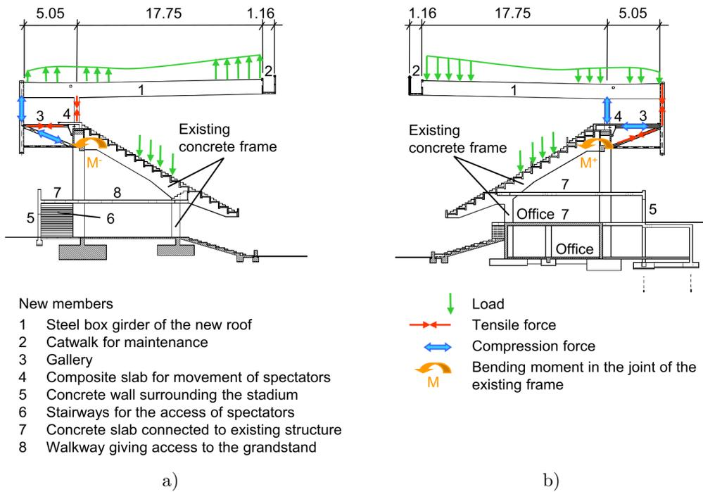
FIGURE 3. Cross-sections after refurbishment and expansion (courtesy of Cesma Ingenieros): a) standard frame; b) frame of main grandstand.
