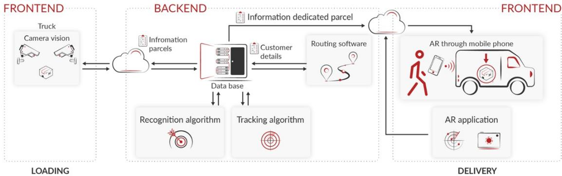
FIGURE 1. System architecture.
