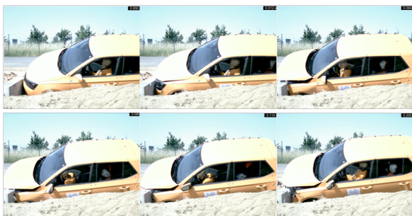
FIGURE 7. Test No. 002 – drainage ditch of a classical construction.
