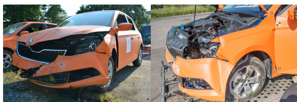
FIGURE 13. Vehicle damage after test No. 002 – drainage ditch with an integrated deformation zone impact.
