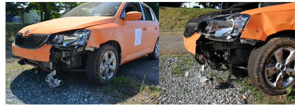
FIGURE 11. Vehicle damage after test No. 001 – drainage ditch with an integrated deformation zone impact.
