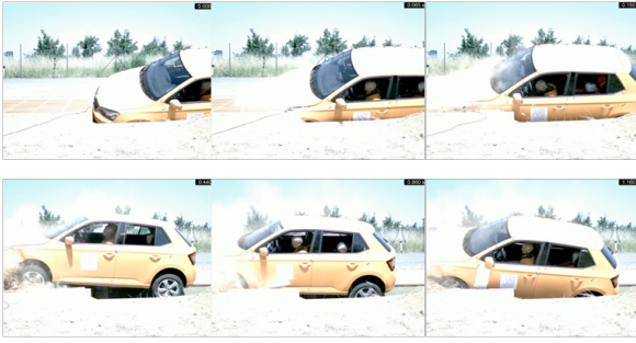
FIGURE 4. A course of the test No. 001 – the vehicle is due to a deformed structure lifted above the barrier.
