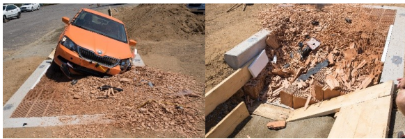
FIGURE 10. Deformation of drainage ditch with an integrated deformation zone after test No. 001.
