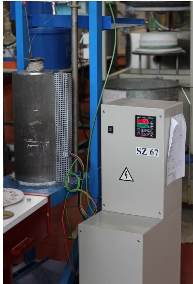
FIGURE 2. Burst-test experimental apparatus
