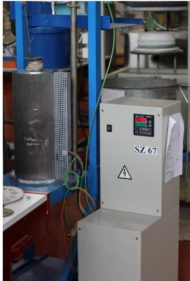
FIGURE 2. Burst-test experimental apparatus
