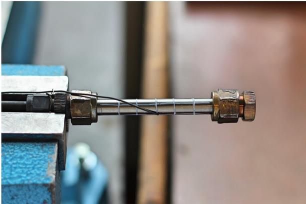
FIGURE 1. Burst-test specimen before exposition in argon
