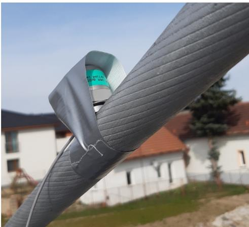
FIGURE 3. Acceleration transducers Brüel&amp;Kjær Type 8344 attached directly to a stay by neodym magnet, the silver tape is used as a security tool only.
