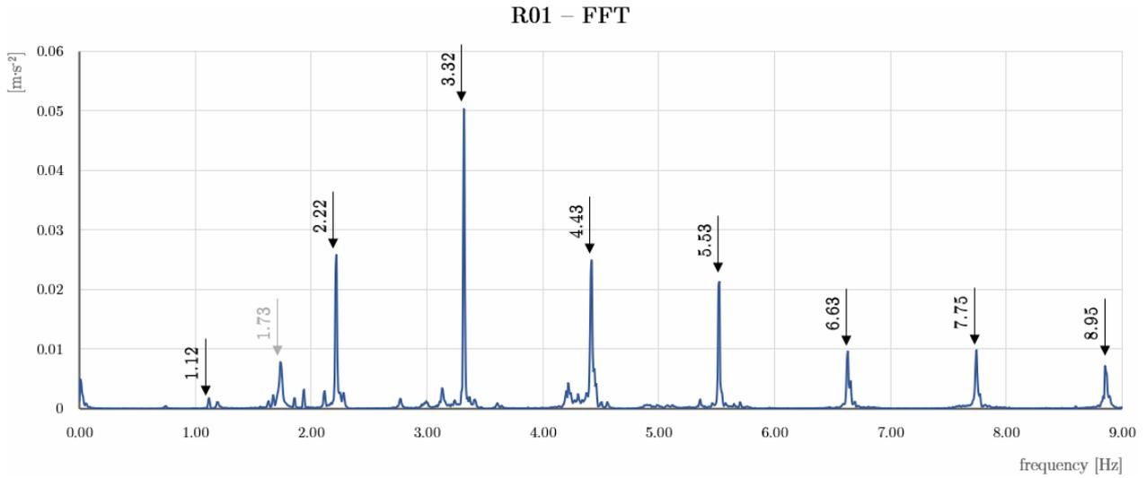
FIGURE 4. Natural frequencies evaluated using FFT – the stay no. R01.
