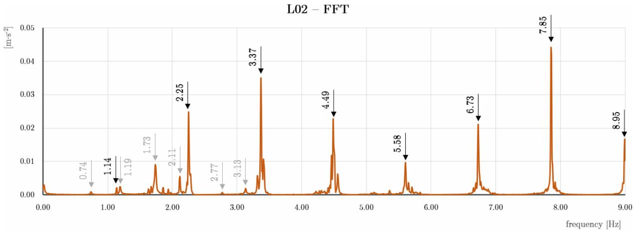
FIGURE 5. Natural frequencies evaluated using FFT – the stay no. L02.
