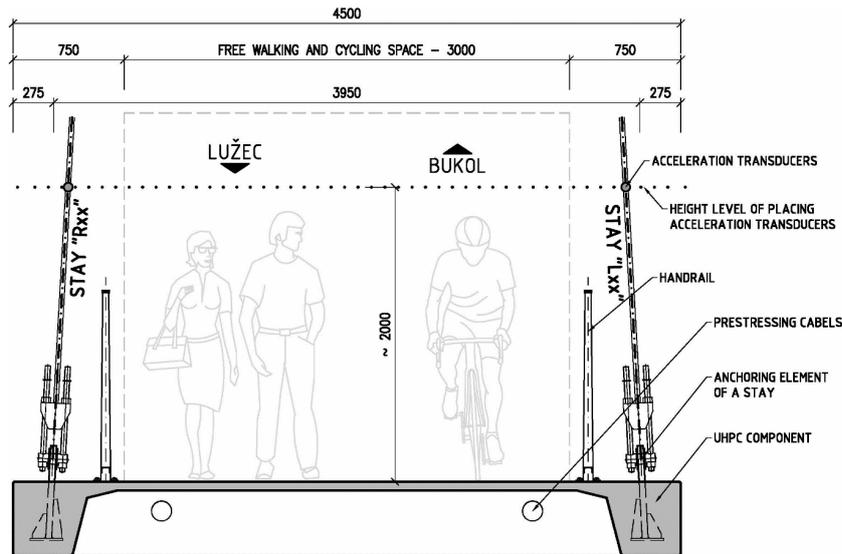
FIGURE 2. Marking the stays – cross section.
