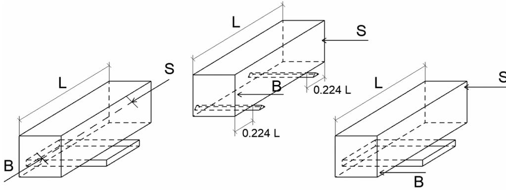
FIGURE 2. Position of the sensor and the impulse hammer on the sample to measure the fundamental frequencies from longitudinal (left), transverse (center), and torsional (right) oscillations; S – sensor, B – impact hammer [11].
