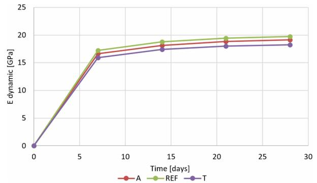
FIGURE 4. Dynamic modulus of elasticity from 0 to 28 days.
