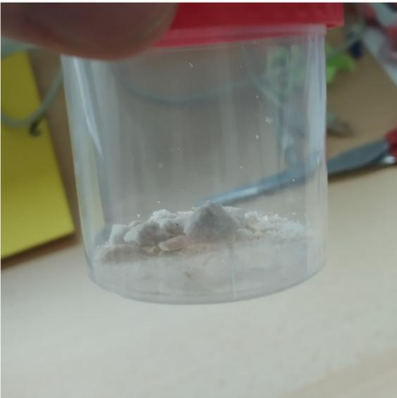
FIGURE 1. Silica sand sample after MICP process.
