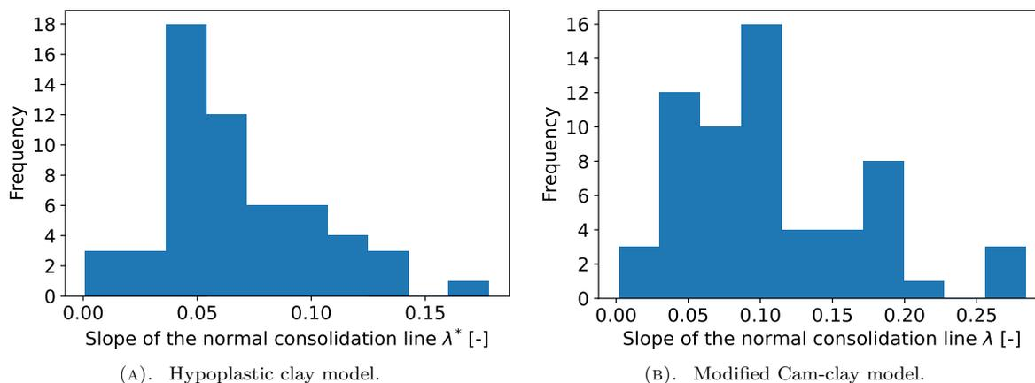
FIGURE 5. Histograms of slopes of the NCL for hypoplastic clay and modified Cam-clay model.
