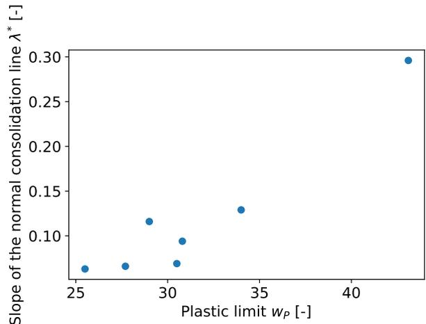
FIGURE 4. Correlation between plastic limit and slope of the NCL assumed in hypoplastic model for clay.
