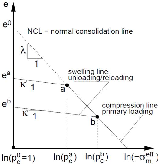
FIGURE 2. Normal consolidation line and swelling line assumed in modified Cam-clay model [2].
