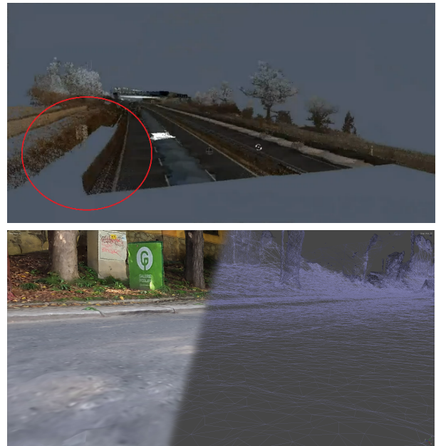
FIGURE 14. The disadvantage of a fixed scanner (in this case, a laser scanner) is the impossibility of collecting data on a site that is not directly visible to the scanner and Example of a model reconstructed from the passage of a measuring vehicle (down).
