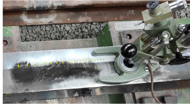
FIGURE 5. Hardness assembly using the Meopta Vickers apparatus on the HEB 140 profile.
