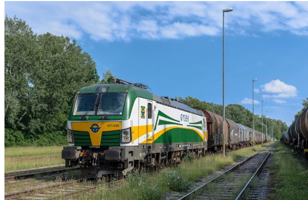
FIGURE 1. Siemens Vectron AC locomotive, which is equipped with last-mile module (small diesel engine), pulling a freight train outside of the electrified track.
