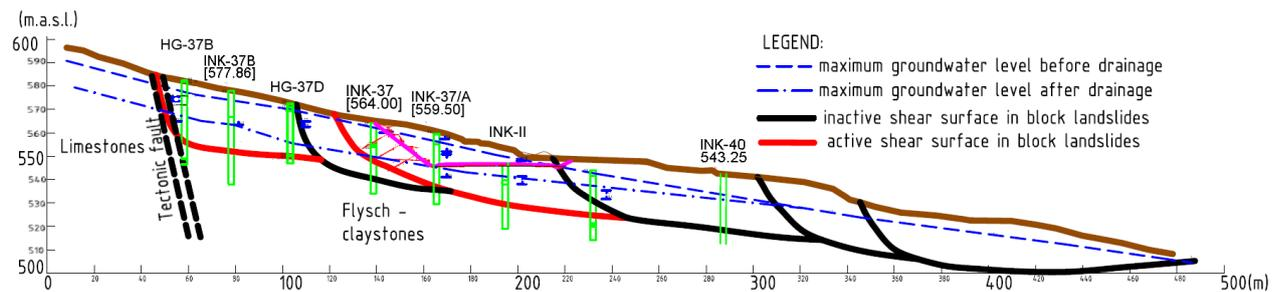
FIGURE 4. Engineering-geological profile of the landslide - model GT-1.
