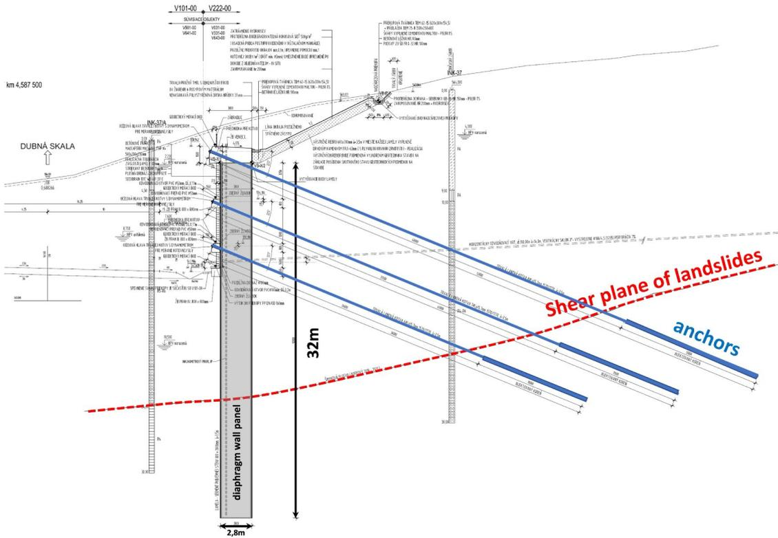
FIGURE 9. Wall cross-section of geotechnical model GT1.
