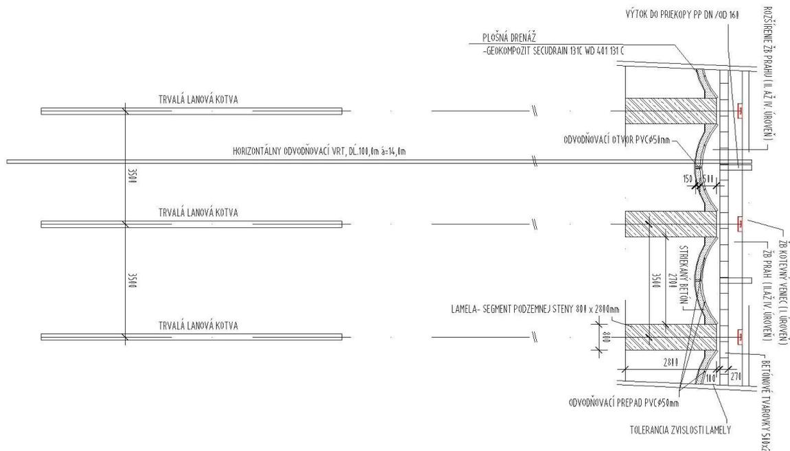
FIGURE 10. Detail of anchor pass-through in panels and counter-vaults of sprayed concrete and HDW.
