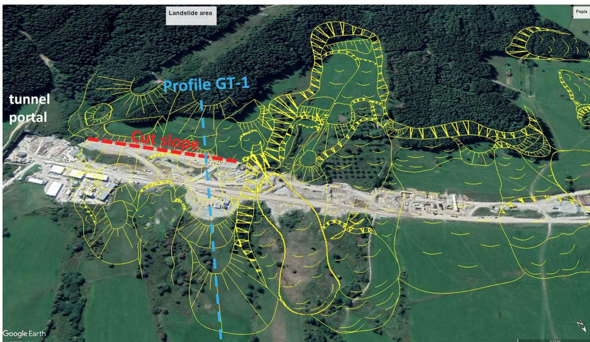
FIGURE 2. Landslide in front of the tunnel portal. The red line is the location of stabilization measures.
