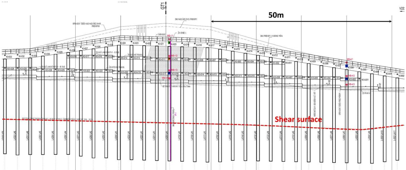
FIGURE 6. Part of the diaphragm retaining wall consisting panel elements in the section of GT1 model.
