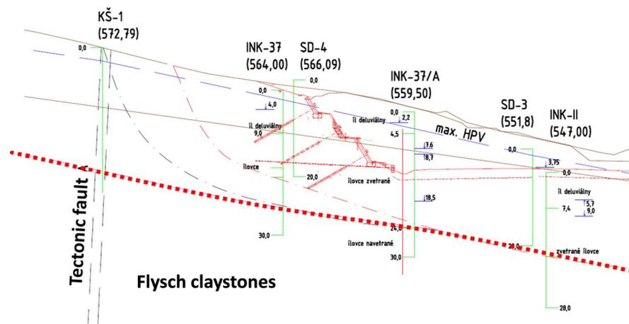
FIGURE 5. The design of the original solution INK-II from 2008 and its location in relation to the determined shear surfaces.
