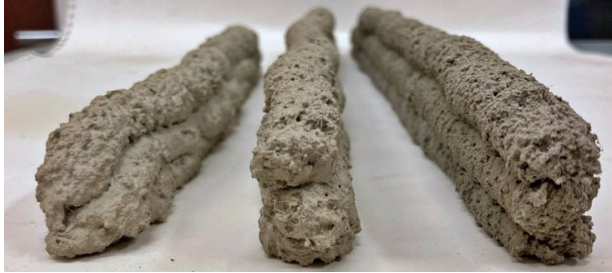
FIGURE 1. Printed layers of cement based material.
