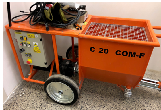
FIGURE 7. Concrete mixture pump with frequency converter.
