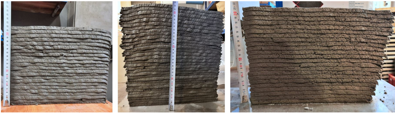
FIGURE 4. Manually printed material with adjusted composition.
