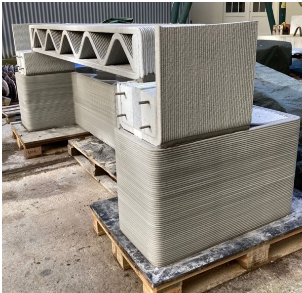
FIGURE 13. Printed wall and truss beam.
