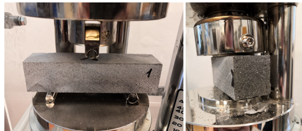
FIGURE 11. Flexural tensile strength test (left) and compressive strength test (right) on 40 × 40 × 160 mm beams.
