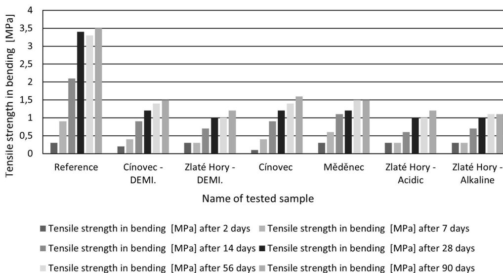
FIGURE 2. Graph showing the tensile strength in bending from Tables 10 and 11 of the tested samples at 2, 7, 14 and 28, 56 and 90 days.
