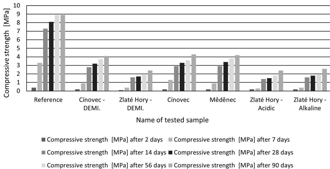
FIGURE 3. Graph showing the Compressive strength from Tables 10 and 11 of the tested samples at 2, 7, 14 and 28, 56 and 90 days.
