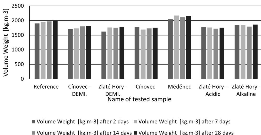
FIGURE 1. Graph showing the volume weights from Table 9 of the tested samples at 2, 7, 14 and 28 days.
