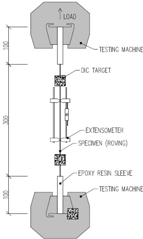
FIGURE 2. Scheme of the tensile test setup.
