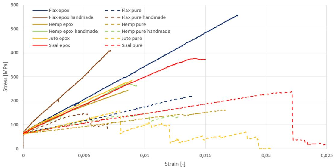
FIGURE 5. Stress-strain chart of representative samples of pure and impregnated samples.
