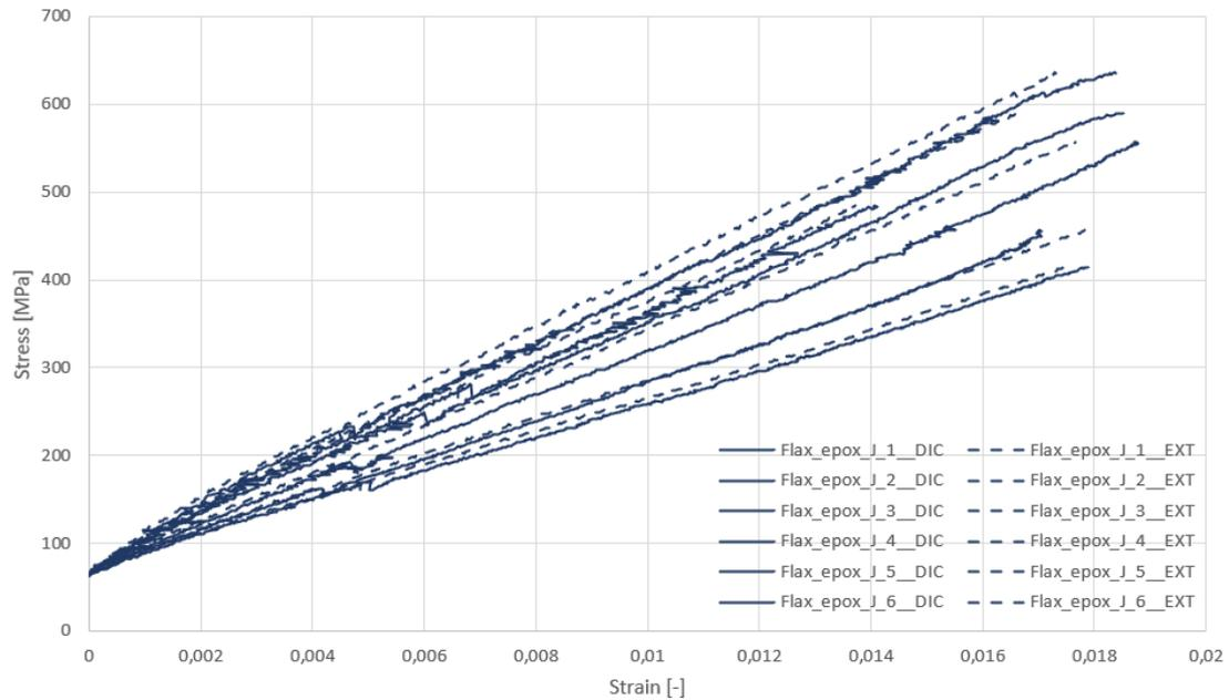
FIGURE 4. Comparison of the flax data measured by DIC and extensometer.
