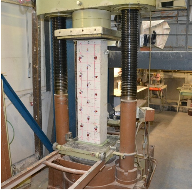
FIGURE 2. Concrete column under load placed in the test press.
