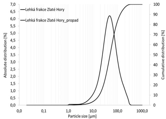
FIGURE 1. Laser granulometry of silicate filler (light fraction) “Zlaté Hory” \*“Lehká frakce” is translated as light fraction in absolute and cumulative distributions.
