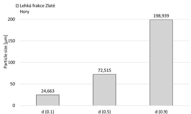
FIGURE 2. Particle distribution of the light component of the “Zlaté Hory” silicate filler \*“Lehká frakce” is translated as light fraction in absolute and cumulative distributions.
