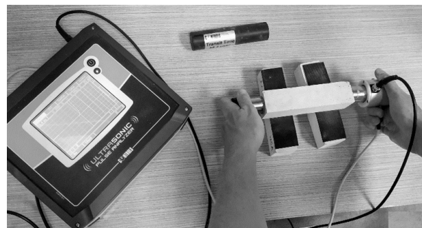
FIGURE 1. The demonstration of ultrasonic signal velocity measurement.
