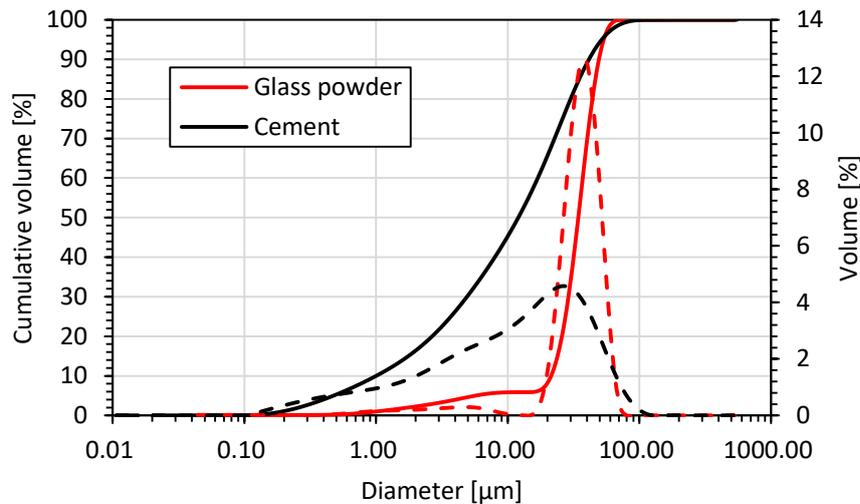
FIGURE 1. Particle size distribution of tested materials.
