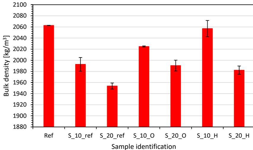
FIGURE 2. Bulk density of test materials with standard deviations.
