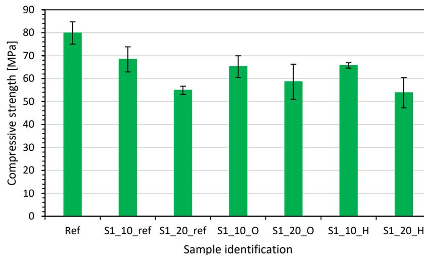
FIGURE 4. Compressive strength of test materials with standard deviations.
