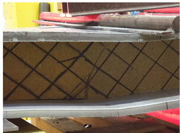
FIGURE 9. Detail of the purenit rib shear failure.
