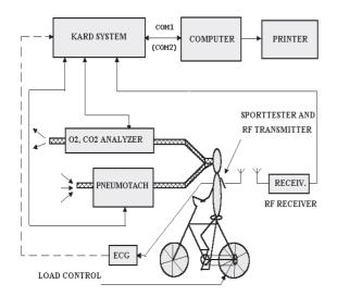
Fig. 1: Block diagram of measuring system for noninvasive CEPT. The cycle or treadmill ergometer can be used.
