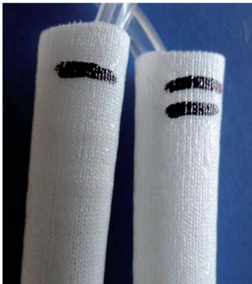
Fig. 1: Samples manufactured from polyester mesh and collagen-based matrix.
