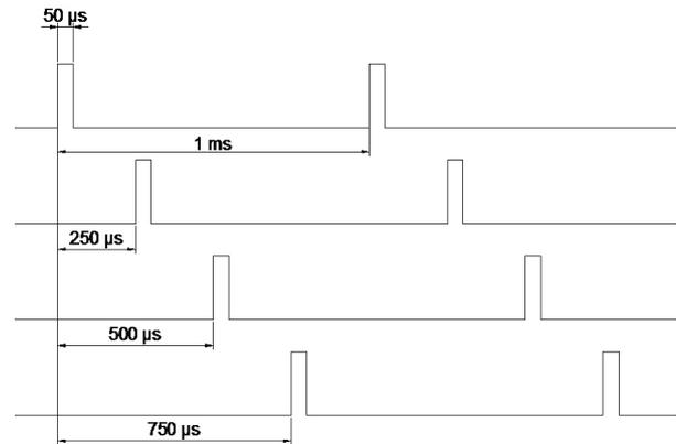
Fig. 4: LED switching timing diagram.
