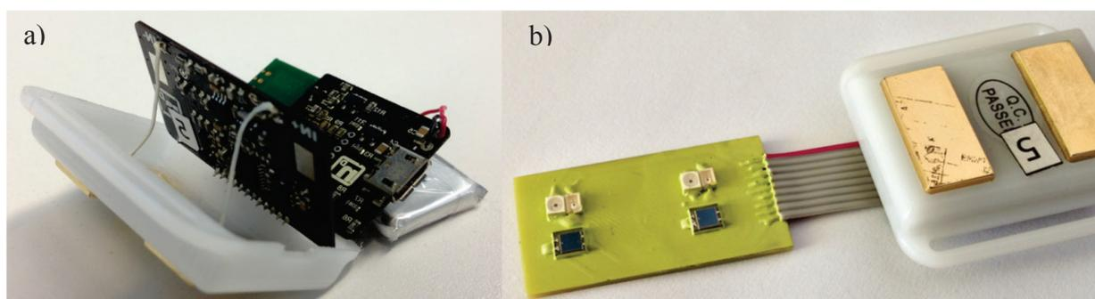
Fig. 1: a) Probe for measuring biosignal from BioSense system. b) Modified probe with integrated pulse oximetry on extension board.
