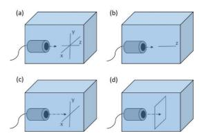
Fig. 3: Examples of scans used. (a) the representtation of xyz axes (b) linear scan along z axis (c) orthogonal cross xy scan (d) planar xy scan.
