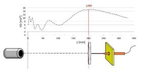
Fig. 2: Experimental set-up shown in correlation with ultrasound field distribution along z axis. LAM: last axial maximum.
