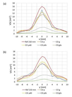
Fig. 7: Orthogonal cross xy scans behind particular culture dishes. Ref 210 mm: reference scan at z = 210 mm. (a) compared values measured on x axis (b) compared values measured on y axis.
