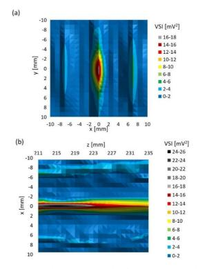
*Fig. 12: (a) planar xy scan behind Eppendorf test tube, (b) planar xz scan behind Eppendorf test tube.*
