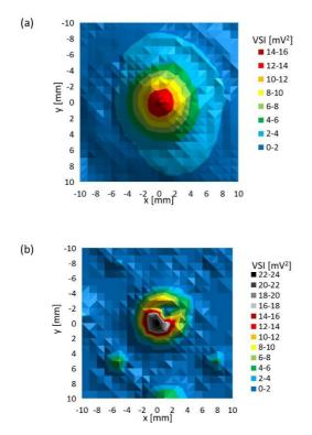
*Fig. 10: Planar xy scan behind particular culture plate (a) 6-well plate, (b) 48-well plate.*
