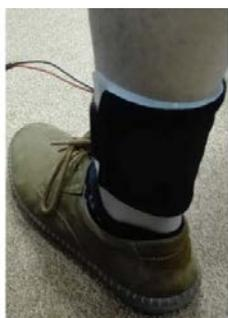
Fig. 3: The  $f$ -TEG module placed on the ankle.
