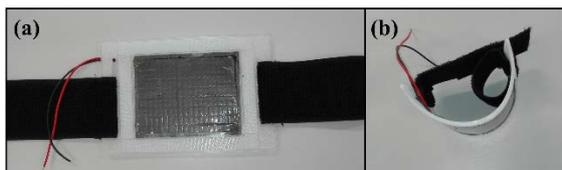
Fig. 1: The *f*-TEG module; TEGway, South Korea. (a) the module in planar position; (b) the module in folded form.
