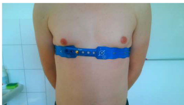
Fig. 1: Subject with size S electrode belt placed in the 5 th intercostal space.
