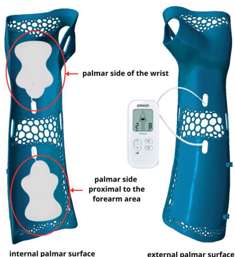
Fig. 1: Proposal of an orthosis with integrated electrode interfaces for electrical stimulation in carpal tunnel syndrome.
