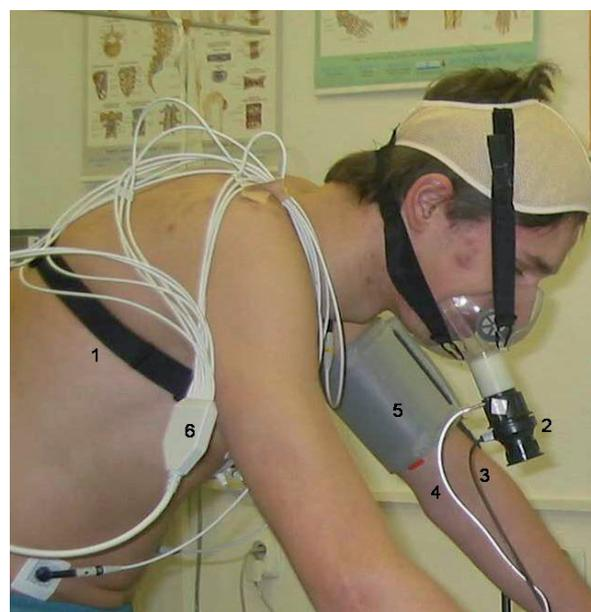
Fig. 2: Equipment for cardiorespiratory values measuring: 1-HR belt (Sporttester), 2-turbine for pulmonary ventilation measuring, 3-cable for ventilation pulses, 4-tube for expired gas samples, 5-cuff for blood pressure monitoring, 6-cable for ECG monitoring.
