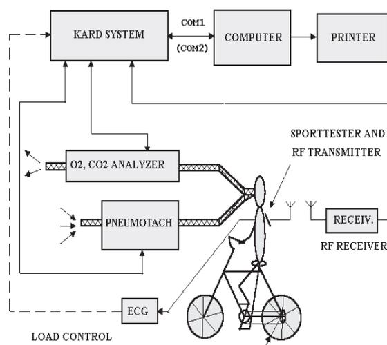
Fig. 1: Block diagram of measuring system for non-invasive CEPT. The cycle or treadmill ergometer can be used.
