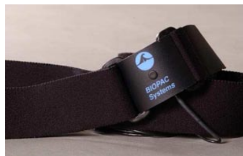
Fig. 2: The sensor for measurement of the tension of the strap.
