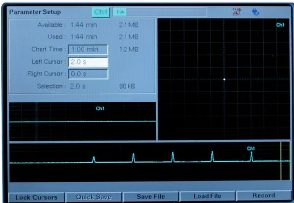
Fig. 6: Dependence of differential response signal on probe movement for  $f = 100$  kHz.
