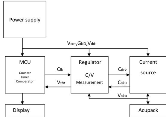
Fig. 2: A block diagram of a testing device conception.
