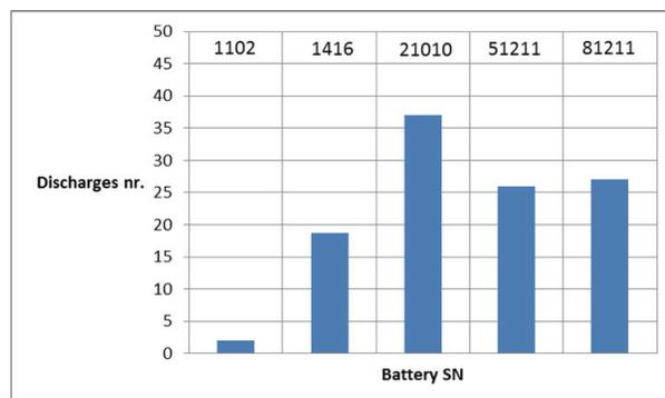
Fig. 4: A comparison between different acu-packs. Amount of discharges depends on the age of acid-lead batteries. Figure shows differences between the extremely old (Nr. 1102), mid age batteries (Nr. 1416, 51211 and 81211) and a new one (Nr. 21010) represented by its serial numbers for the database.
