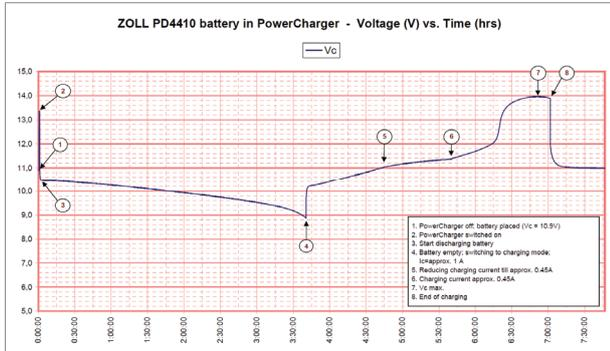
Fig. 1: The description of the voltage dependence on time for charging the battery in the charger ZOLL. 1 – acu-pack placement into the charger; 2 – power charger switched on; 3 – discharging battery started; 4 – battery empty – switching to charging mode, current approx. 1 A; Reducing charging current to approx. 0.45 A; 7 – maximum battery voltage; 8 – end of the charging cycle.
