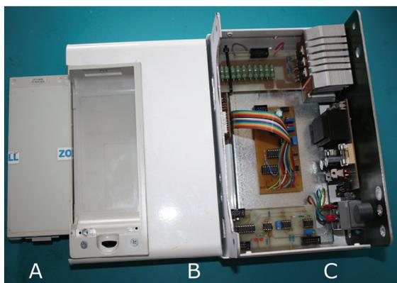
Fig. 3: Mechanical conception of the testing device. A - an original ZOLL lead-acid battery pack, B - a battery pack berth (original ZOLL), C - metallic box with the printed circuit boards.
