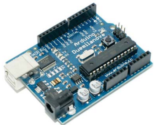
Fig. 3: Development board Arduino Duemilanove with microcontroller ATmega328P.
