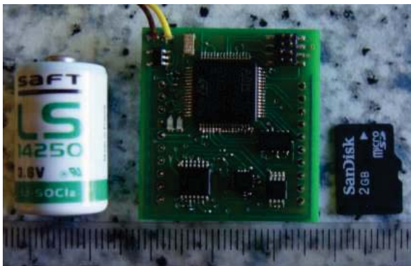
Fig. 1: The ActimedARM (center), a \mu SD card (right) and a battery (left).
