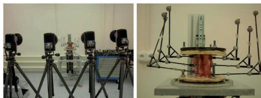
Fig. 6: The recording device on the left. The markers mounted to the sample on the right.
