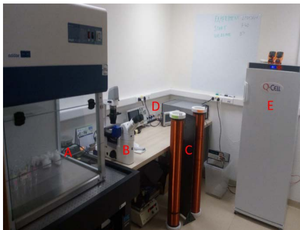
Fig. 1: Experimental set-up. A – PCR box, B – optical microscope, C – two identical MF applicators, D – EMF excitation system, which incorporates signal generator, amplifier HUBERT A 1100-16 (DC-1MHz), and digital multimeter for electric current monitoring, E – incubator Q-cell.
