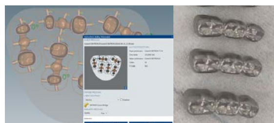
Fig. 3: Software interface for setting up the support and subsequently produced samples by CNC milling.
