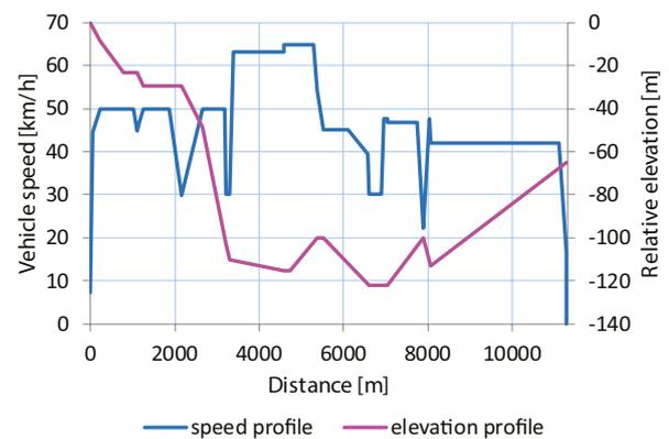
**FIGURE 8:** Optimized speed and elevation profile on simulated route.
