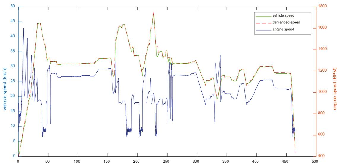
**FIGURE 9:** Results of drive cycle simulation for engine predictive model training.
