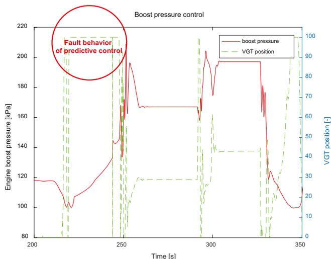
**FIGURE 5:** Result of predictive engine boost control with fault behavior in acceleration phase.
