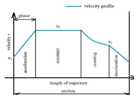
**FIGURE 7:** Velocity profile and driving phases in each section.
