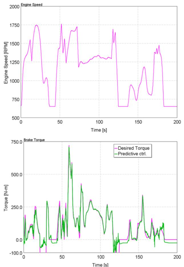
FIGURE 11: Result of simulation of WHTC – engine speed (left) and engine brake torque (right).
