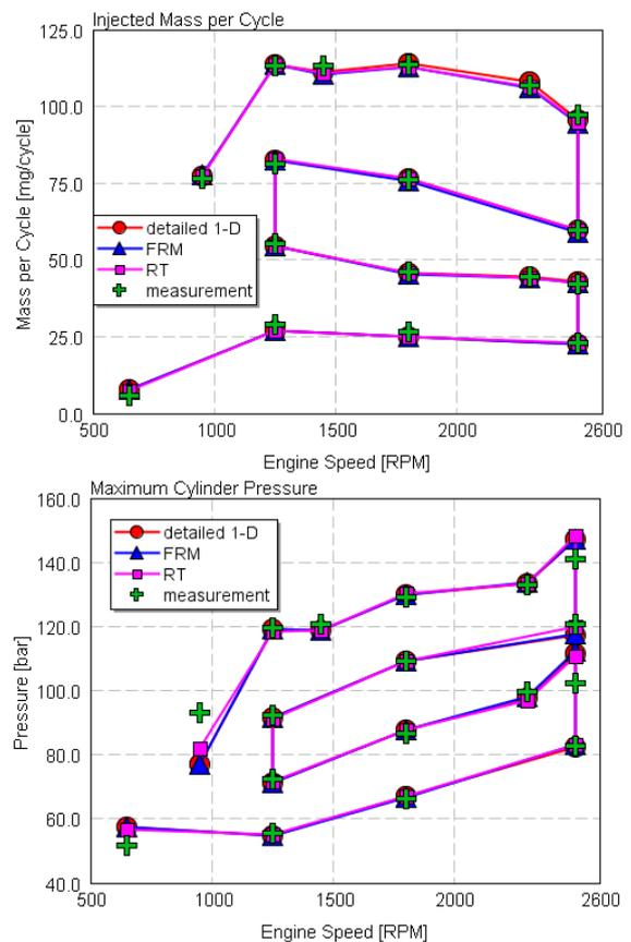
FIGURE 2: Results comparison of detailed 1-D model and FRM model with measured data – injected fuel mass per cycle (upper) and maximum cylinder pressure (lower).
