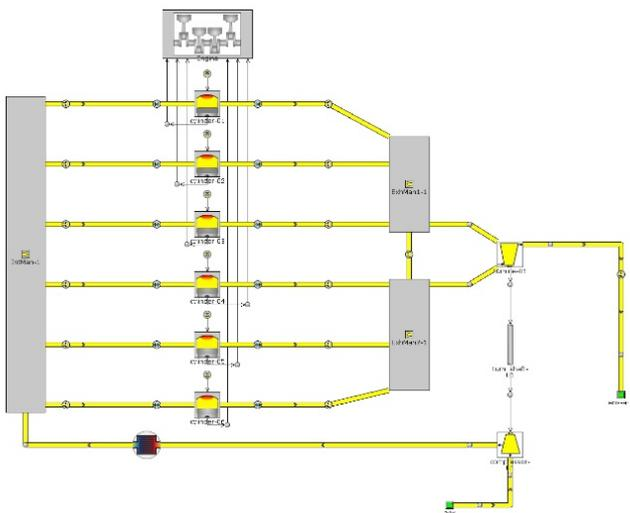
FIGURE 1: Fast Running Model of engine in GT-Power.
