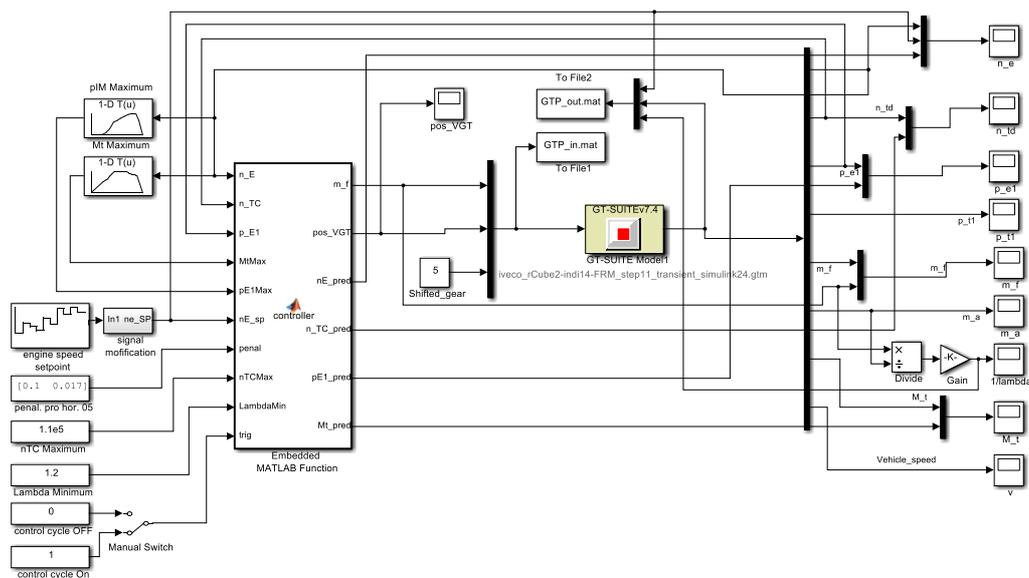
FIGURE 10: Simulink / GT-Suite co-simulation (closed-loop control).
