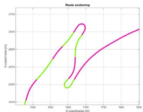
**FIGURE 6:** Possible velocity limits along the route (left) and route trajectory sectioning by the maneuvers classification (right).
