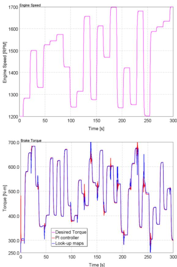
**FIGURE 4:** Predictive engine model training with random step signal – engine speed (left) and engine torque (right).
