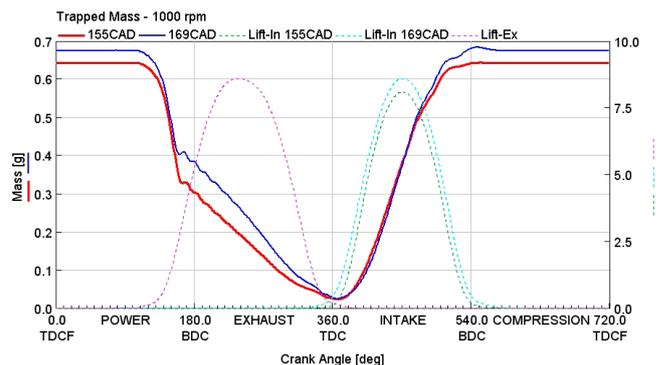
**FIGURE 11:** Total mass flow through valves
