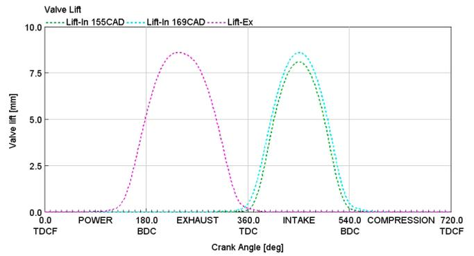
**FIGURE 7:** Valve profiles
