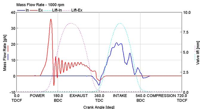
**FIGURE 8:** Mass flow rate through valves– 169CAD
