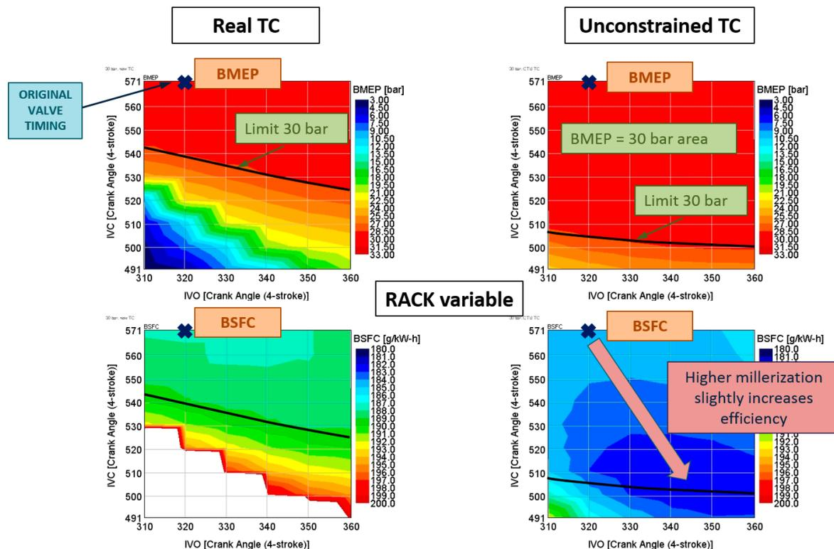
FIGURE 3: Comparison of turbochargers
