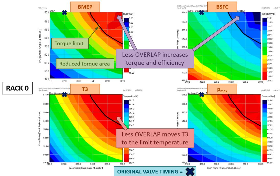
**FIGURE 6:** Results of valve timing sweep
