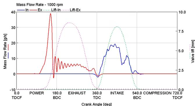
**FIGURE 9:** Mass flow rates through valves– 155CAD
