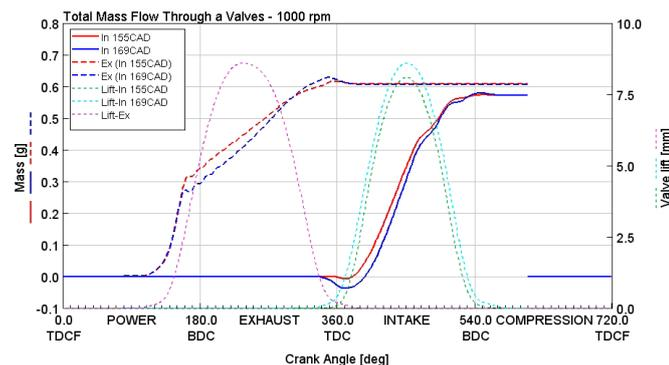
**FIGURE 10:** Total mass flow through valves
