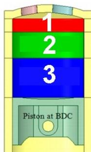
**FIGURE 14:** Cylinder temperature zones, see [16]
