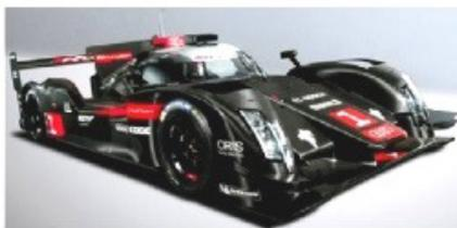
**Audi R18 e-tron Quattro** has Diesel V6 with electric turbocharger rear, two electric motors at front axle and flywheel in cabin
