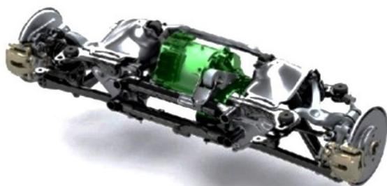
**FIGURE 6:** Hybrid4 models Peugeot / Citroen uses an electric motor connected to the rear axle via a gear and a clutch. Vehicles with this drive may drive in pure electric mode, hybrid mode or as a 4x4
