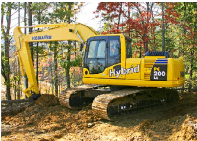
**FIGURE 14:** Excavator scoops up earth and turns the tower to the place where the earth is deposited. The drive of rotation is electrical, when rotation is braking the energy is stored in a super-capacitor and subsequently is used for rotation in the opposite direction.
