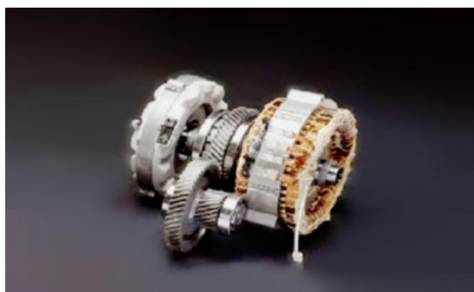
**FIGURE 5:** Toyota Hybrid Synergy Drive uses a planetary power divider, has no clutch or gear shifting members and continuously varies the gear ratio as a CVT
