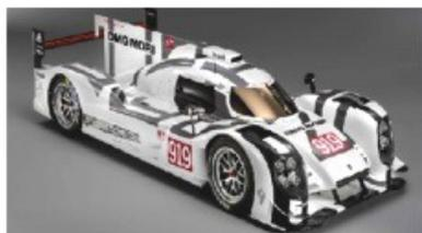
**Porsche 919 Hybrid** has turbocharged engine V4 rear with system of energy regeneration from exhaust gases, electric motor at front axle and battery in cabin
