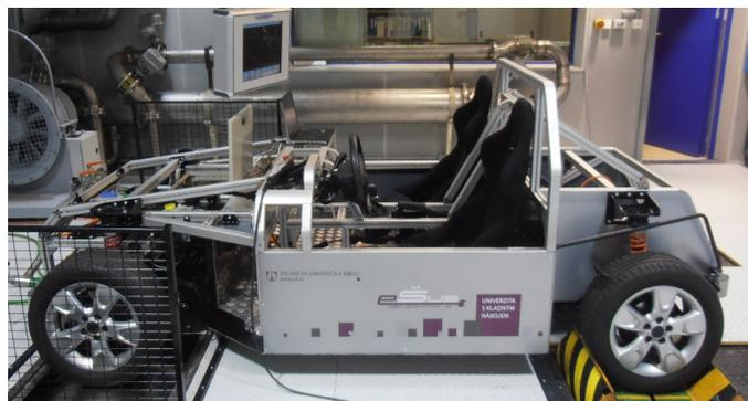
FIGURE 1: Experimental electric vehicle eŠus Gen2.
