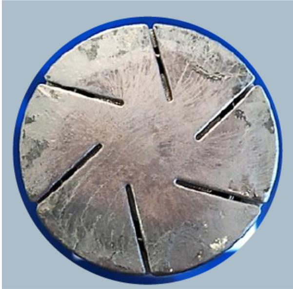
Figure 2. Picture of one contact surface of the opened VI after all current interruptions.
